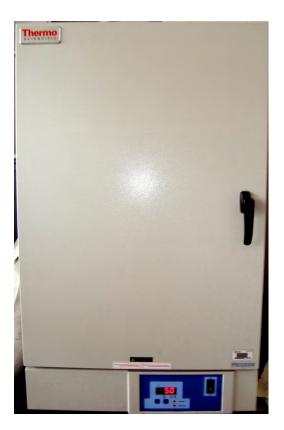
Figure 2: Oven set to 50 to 60 degrees C for drying out the collected sample placed in Pyrex dishes
