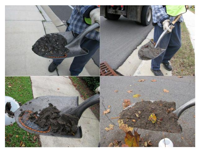
Figure 1: Visual indication of moisture content variability that can be observed in collected samples of solids that have been recovered during the MS4 study (can vary from dry to wet (top left)
