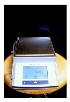
Figure 5: Top-loading weighing scale ('zero' scale before using)
